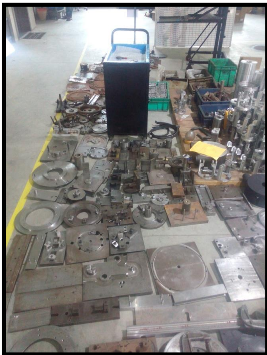
Fig.1 Before SMED - No Rack for fixture Fig.2 Fixture Rack with Identification
