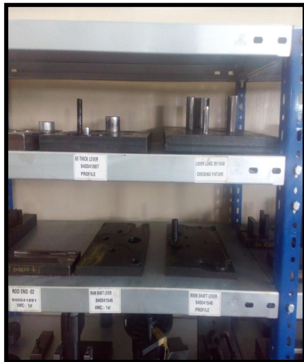
Fig.1 Before SMED - No Rack for fixture Fig.2 Fixture Rack with Identification
